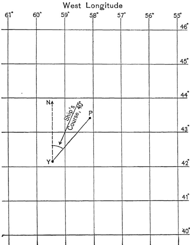
FIG. 1. — Dead Reckoning. (Diagram not drawn to scale.)
