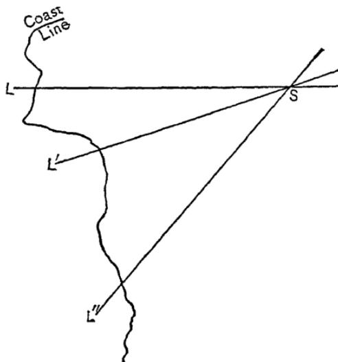
FIG. 10. — Ship's Position by Cross Bearings.
