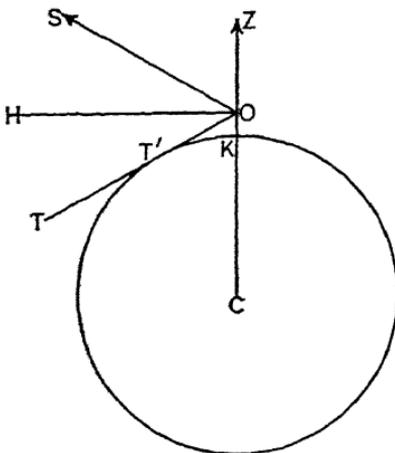
FIG. 17. — Dip of the Horizon.
