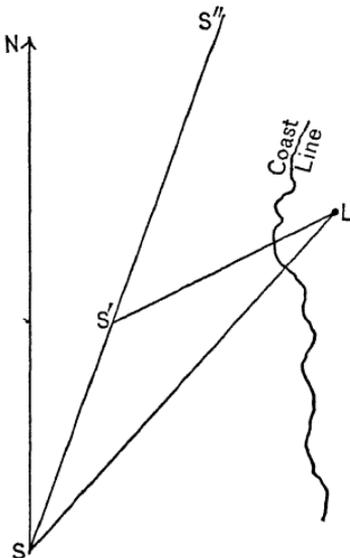
FIG. 9.—Ship's Position by Two Bearings.
