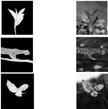
Figure 1: The results of edge detection above. The first column is outputs of the learned PDEs. The second column is input images
